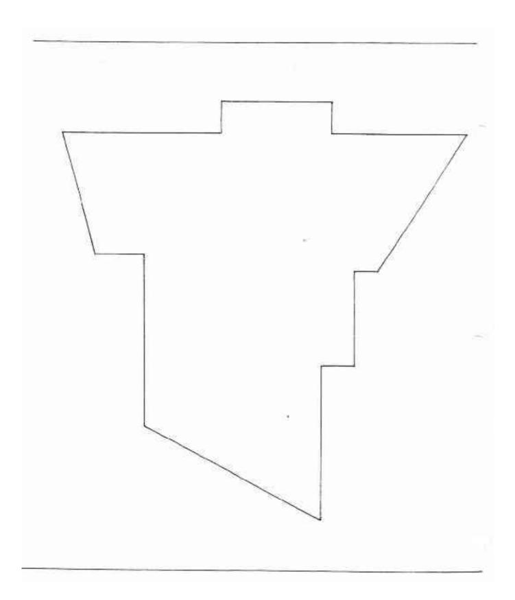
On the Plan below draw in the position of the hips, ridges and valleys and on the line draw the elevation of the roof pitched at 30 degrees.
